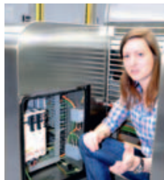
Anne Gerlach, ALUS Development/GEA Lyophil, explains the structure of the PacDrive automation solution with shared power supply.
