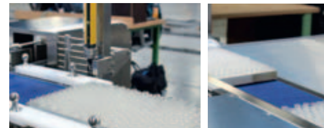
The vials, shown here on optional tablets, approach the unit and are then pushed across the bridge by a slide into the freeze dryer. The process is reversed after the freeze drying process is complete.
