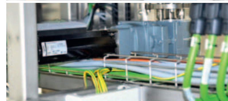
The Lexium 62 ILM servo drives, connected with the distribution boxes and hybrid cables, are located in the base of the ALUS, outside of the hygiene-critical area.
